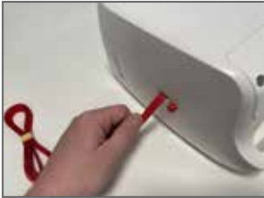
1. Activate the emergency stop by pulling the red ribbon.
