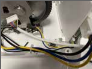
3. Slide the cable holder and tighten.
