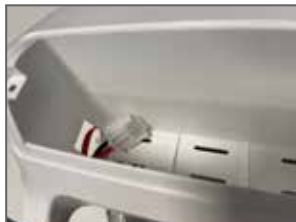
7.2. Remove the top cover (take note of the cables and the connectors)
