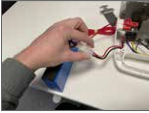
1. Remove the top cover. Connect the battery.
