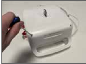
2. Remove the battery cover with the Allen key.
