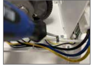
2. Loosen the screws holding the cable.
