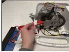
2. Deactivate the emergency stop by pushing the red button.
