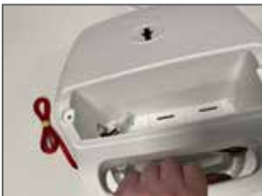
7.1. Remove the top cover (take note of the cables and the connectors)
